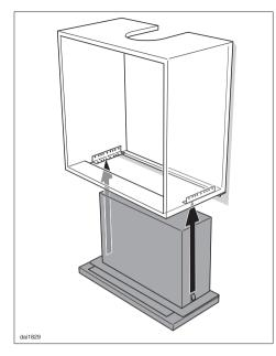
Lift the appliance up into the housing from below until it engages in the brackets.
